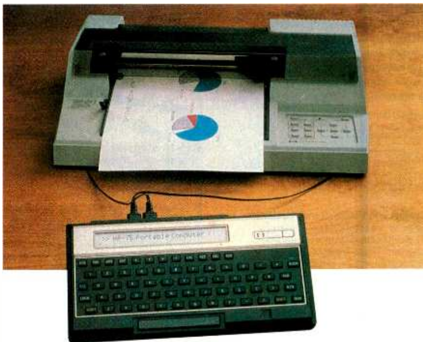
The HP-75C connected to a Hewlett-Packard plotter through the HP Interface Loop.
