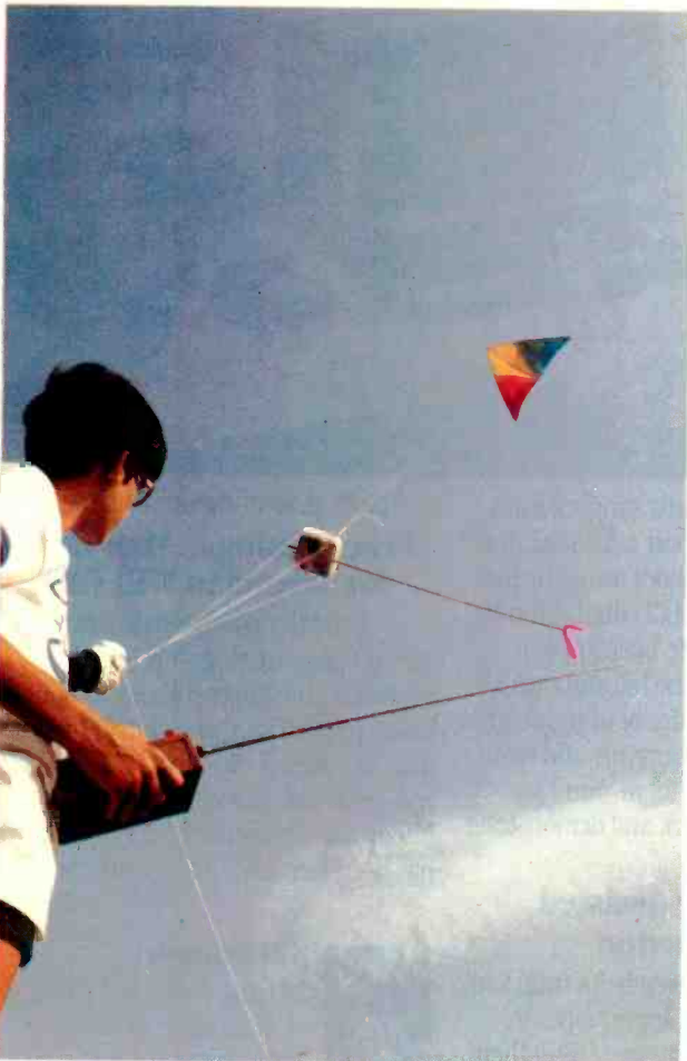
This 3' x 6' kite can tow a 12-oz RC disc camera package to an altitude approaching 1000 ft.
