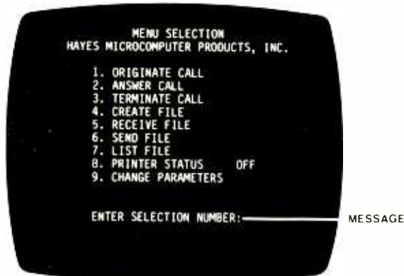
Fig. 2. When the system is ready and booted, the Hayes Terminal Program displays this menu.
