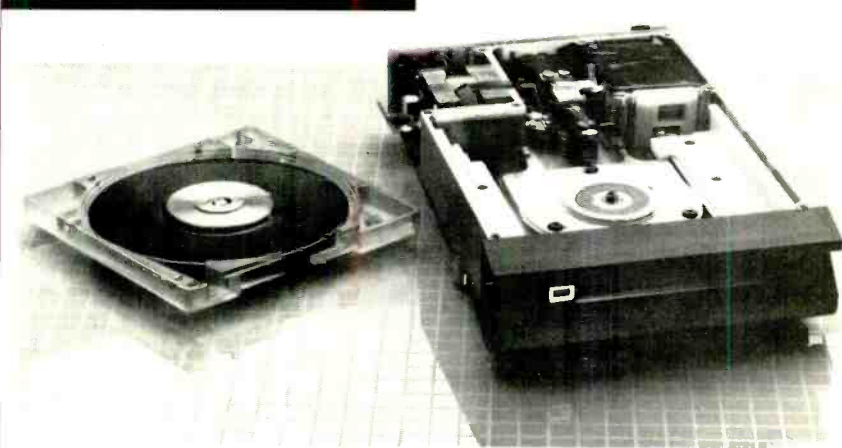
The Syquest SQ306 hard disk drive uses removable 3.9" cartridges.
