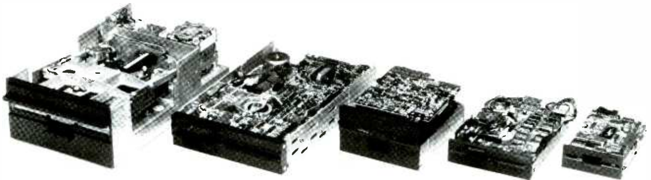
The shrinking world of disk drives is shown by a conventional 8" at left, followed by a half-size 8", conventional and half-size 5 1/4", and 3 1/2" drive at far right.
