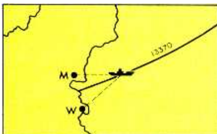
Fig. 1. A line of position (LOP) plotted between two Loran-C stations.
