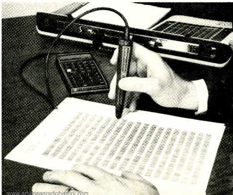
Hewlett-Packard's bar code-reading Optical Wand (HP-82153A) plugs into the HP-41C computer.
