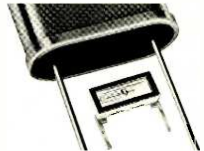
Statek's miniature quartz crystal between leads of an HC-33 can.
