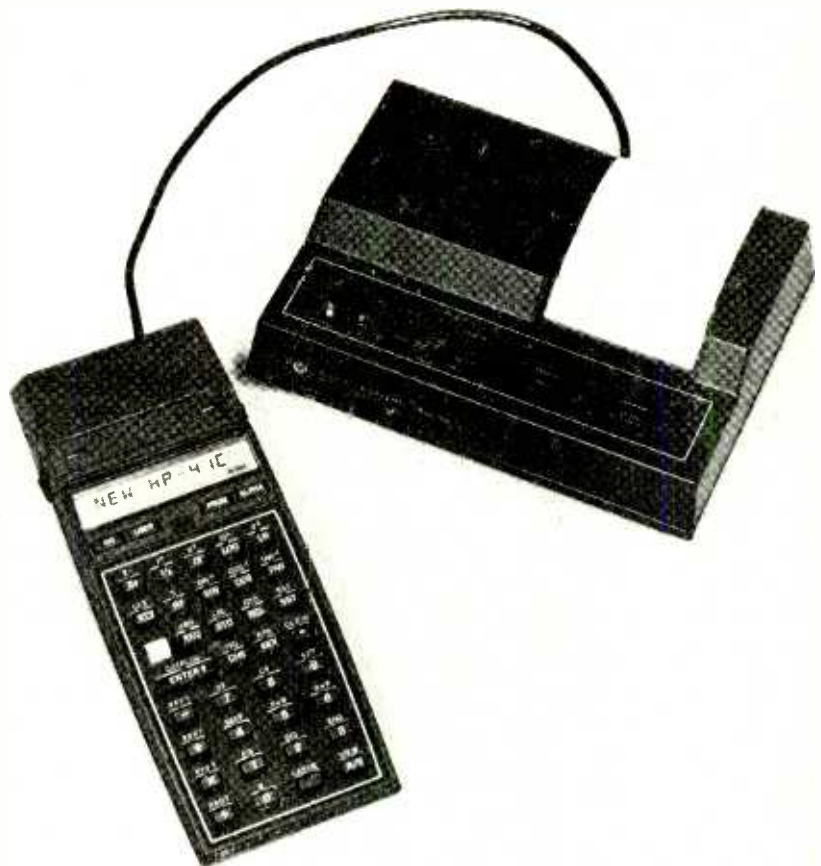
The HP-41C shown here is generating the function \sin x . The output, with the curve, is shown on the printer.
