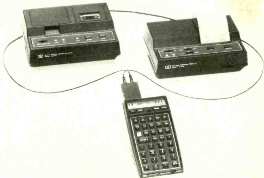
The HP-IL Interface Loop gives the HP-41 mass memory and printing capability with a Cassette Drive and Thermal Printer/Plotter.
