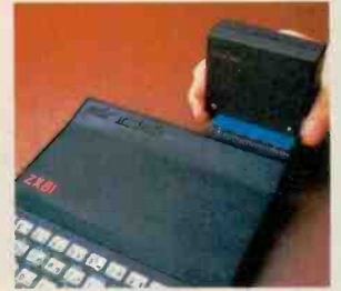
16K MEMORY MODULE: Like any powerful, full fledged computer, the ZX81 is expandable. Sinclair's 16K memory module plugs right onto the back of your ZX81. Cost is $99.95, plus shipping and handling.
