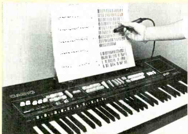
Casio CT-701 electronic computerized player piano uses a tune printed in bar code.
