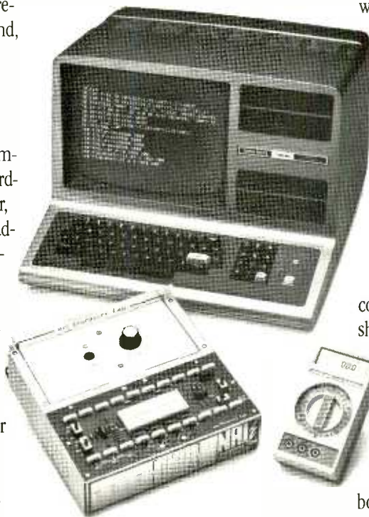
Training includes the new TRS-80 Model III microcomputer, 6-function LCD Beckman multi meter, and the NRI Discovery Lab with hundreds of tests and experiments.
