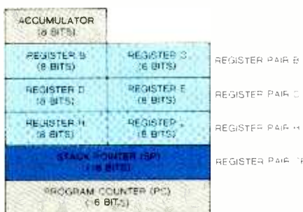
Fig. 18. The 8080 has seven 8-bit general-purpose registers and two 16-bit registers.
