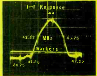
Fig. 4. Factory alignment is good except for placement of lower audio adjacent channel marker, which could be closer to response curve.
