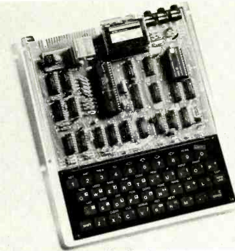
Photo of the ZX80 with its cover removed shows the compact assembly that was used to achieve its small size.
