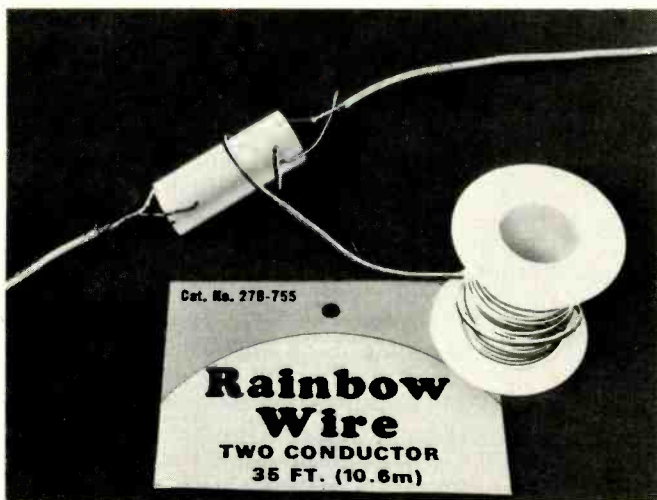
Fig. 6. Two of the antenna's wire elements have been connected to the plastic form and the Rainbow Wire attached.
