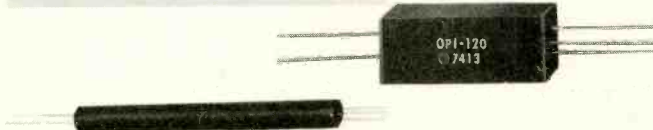
Three TRW Optron isolators: above right, 15-kV rating with CTR of 20%; above left, 50-kV, 10% CTR; at right, 6-kV, 400% CTR.
