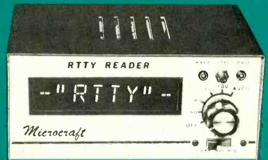
Microcraft's RTTY Reader uses a microprocessor to handle Baudot at four speeds or ASCII and display it on an eight-moving-character readout.
