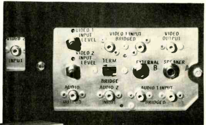
At left is RCA's ColorTrak Video Monitor Model VEM575. Above is a view of the input and output jacks located on the rear panel.
