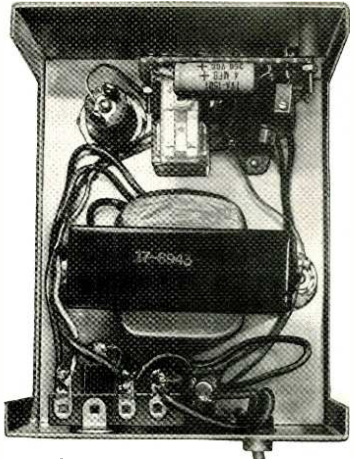
Interior photo of the prototype regulator. Components can be mounted on pc or perf board.
