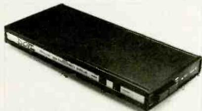
six-line business phone. It features a separate power supply and a mode switch that allows the user to monitor whether voice or data is being transmitted. \$199. Address: Novation, 18664 Oxnard St., Tarzana, CA 91356.
