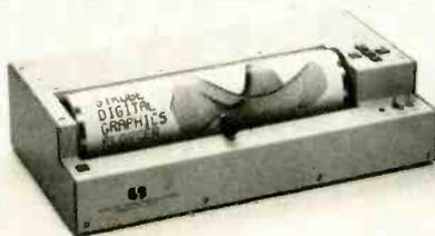
Strobe's Model 100 combined alphanumeric and graphics plotter is a drum-type system that uses 4-phase stepping motors to achieve 0.004-inch (0.1 mm) motions on each axis. It accepts any 8½" by 11" paper and a variety of conventional pens. An interactive digitizing mode enters pen data
