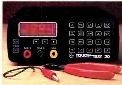
Nonlinear Systems' new 3 1/2-digit LED "Touch Test 20" multimeter uses modern touch switches on its front panel in place of mechanical switches to control function, range and power. In addition to traditional DMM tests, it includes capacitance, temperature, and conductance measurement capabilities. Test parameters
