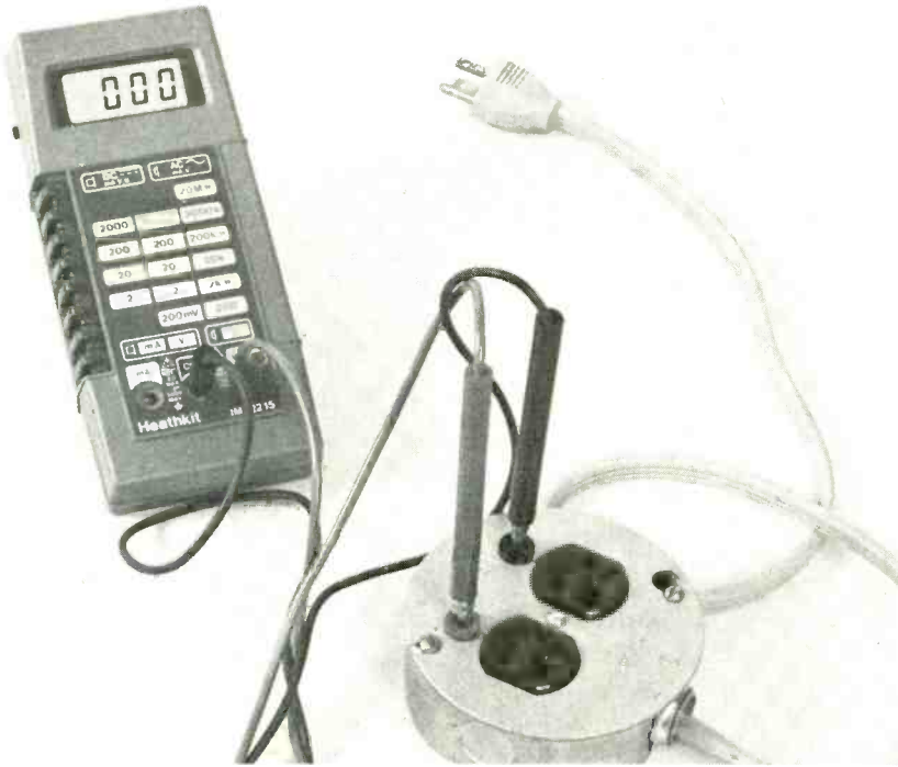
Fig. 5. To measure ac current, the shunt can be coiled inside a conventional ac outlet box and the two tip jacks mounted on the top plate.
