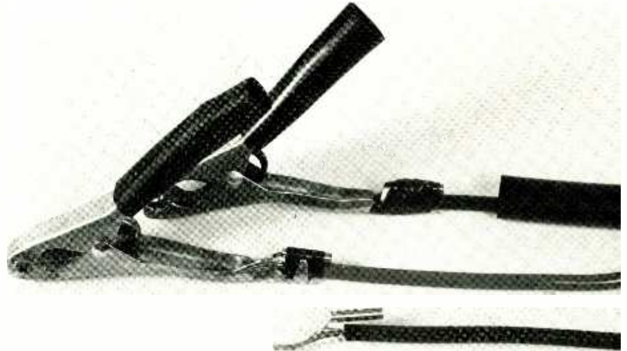
Fig. 3. Assembly of the tip jack and shunt cable to the clamp. After soldering, the large plastic sleeve is placed over the joint and clamp handle.
