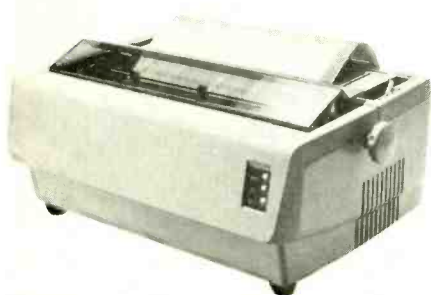
The Starwriter Daisy-wheel printer provides 136 columns of pica type.
