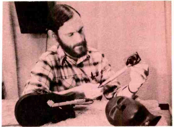
Artificial head used at AR and many other laboratories is made by Neumann, German manufacturer of professional condenser microphones. Units are built with specially designed coupling chambers between ear canal and microphone capsule, to match electrical output as closely as possible to acoustical signal at human eardrum.
