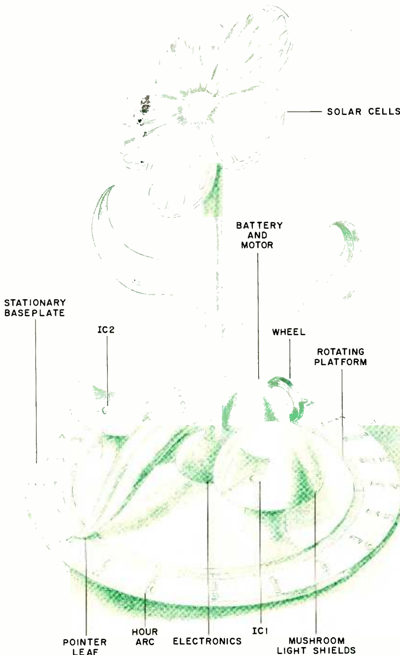
In this design, a flower and mushrooms made of plastic hold the solar cells and light sensors with a leaf for a pointer.
