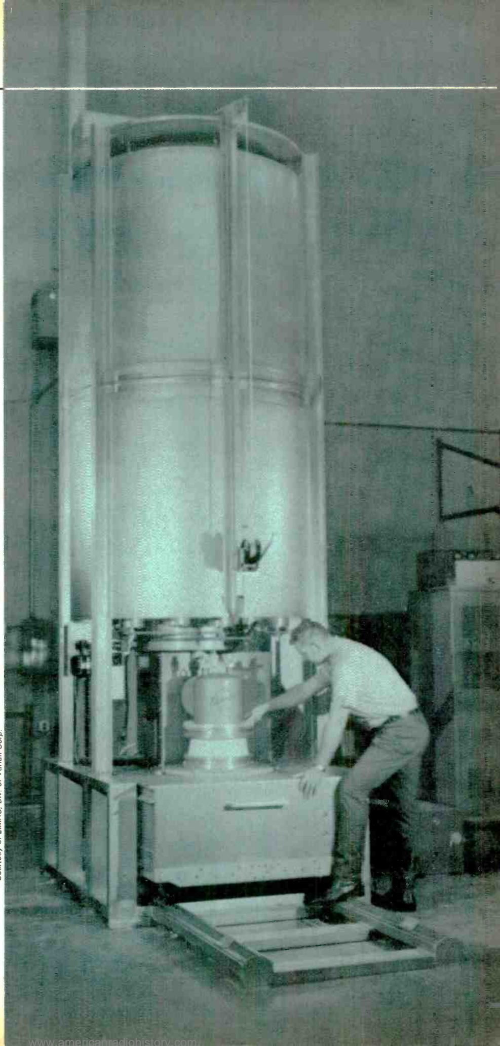
Fig. 3. Giant power vacuum tube typically found in longwave transmitters. This water-cooled tetrode weighs 175 lb (80 kg) and has a rated plate dissipation of 1.25 megawatts!
