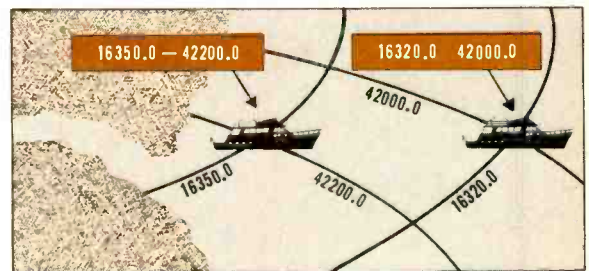
Fig. 2. Radiolocation by LORAN-C signals and charts. A special receiver directs the user to two curved "lines of position." The intersection of these lines pinpoints receiver location.
