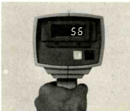
The speed is flashed on the large LED display and is shown in miles per hour.
