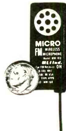
The Micro FM Wireless Mike has a range of over 300 ft. and transmits through any standard FM Radio.
