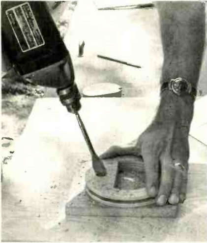
Fig. 6. Drill shaft hole with wood bit, tilting it away from D cutout by about 18 degrees.
