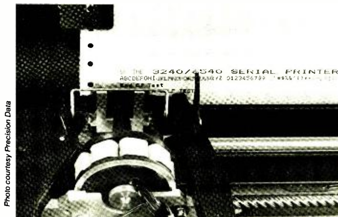
Matrix printhead is used exclusively in nonimpact and in some impact printers.
