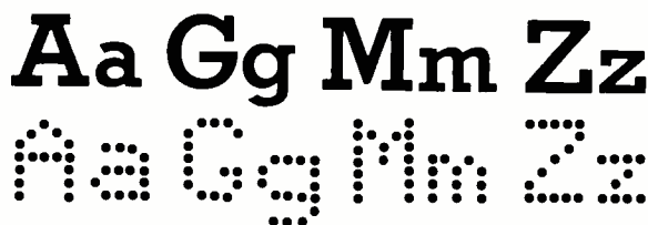
Dot-matrix characters (bottom) may be more difficult to read than solid characters (top).
