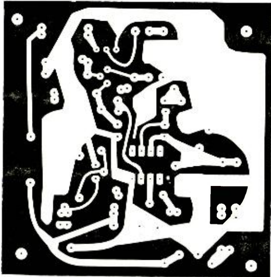
Fig. 3. Actual-size etching and drilling guide is shown at left. Component placement guide is above.
