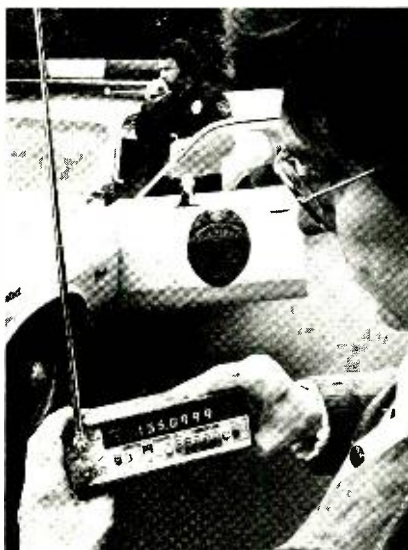
The 1911A multicounter makes accurate field transmitter frequency checks easy with the optional battery-pack and whip antenna.
