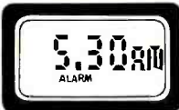
When the alarm's set, "ALARM" appears. To check for the time, touch the alarm button.
