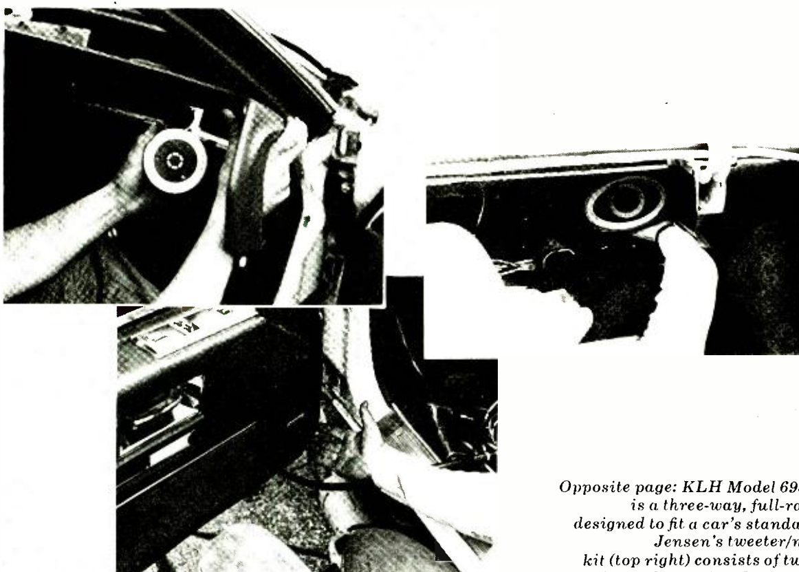
Here's an example of how different speakers can be used to enhance car stereo sound, using Kriket "Audio Separates" drivers. Dome tweeters are installed high in dash (left); 5-inch midrange/woofers mount in front doors (center); Domaxial™ biamplified full-range speakers mount in trunk (right).
