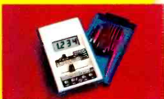
Removable cover stores test lead set furnished as part of the unit.
