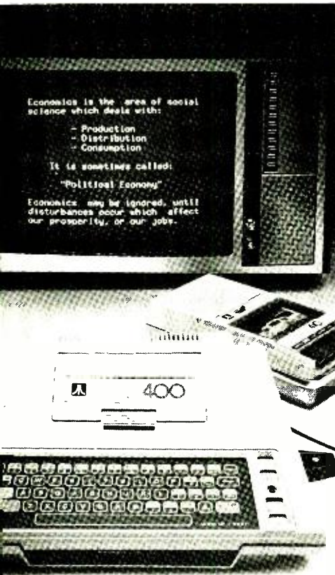
The Atari-400 personal computer uses a 6502 CPU, 8K of RAM and 8K of ROM. Keyboard is a 56-key Monopanel with touch-control points.
