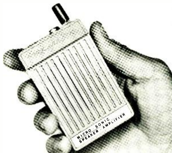
Fig. 1. Portable battery powered amplifier suitable for monitoring modulated light. Plug inserted into microphone jack incorporates a miniature silicon photodiode.
