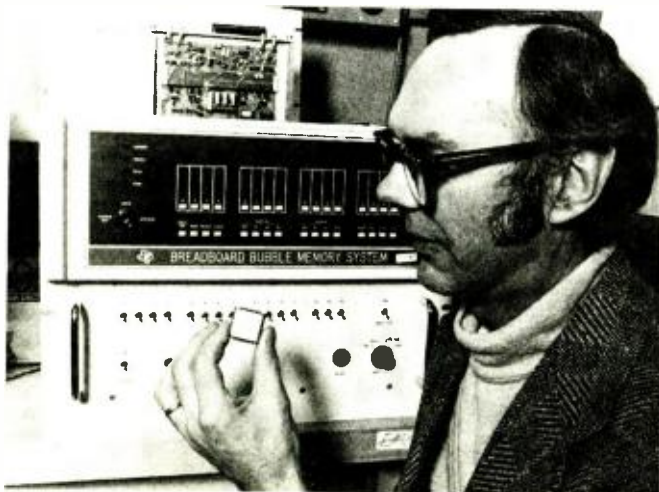
The bubble memory held by an engineer contains two garnet chips and stores 250,000 bits. Sixteen chips are in system at rear, which was developed for the Air Force by Texas Instruments.
