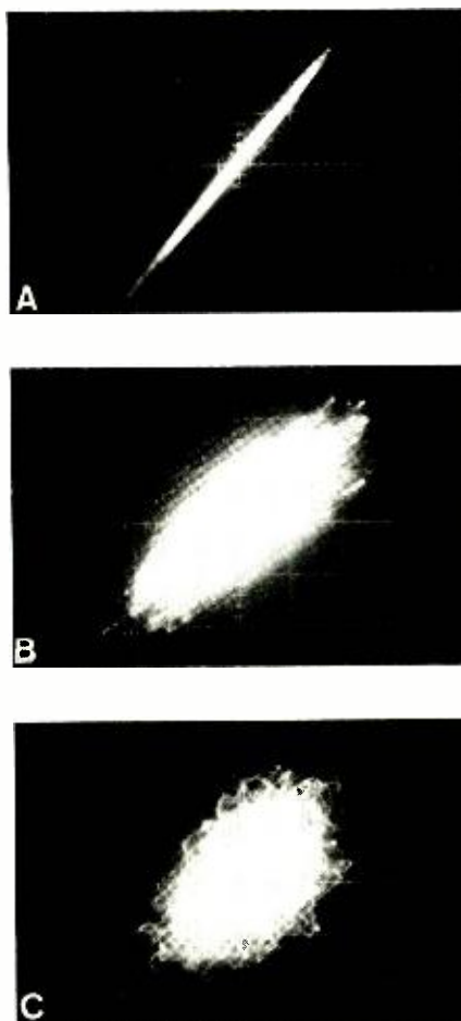
Fig. 2. Some time delay components have coherent (in-phase) outputs (A) as in Bozak Model 902. Others, such as the Advent Model 500, are partially coherent (B). Still others, such as the Audio/Pulse Model One, are non-coherent (C).
