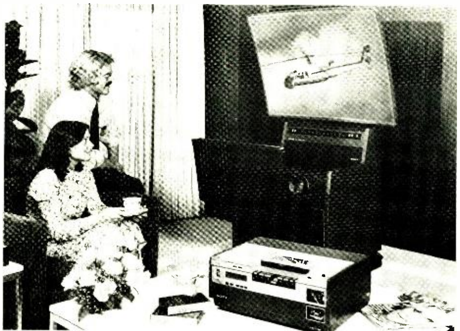
Self-contained type of projection TV, such as the Sony Corp. model above right, uses mirror to reflect enlarged TV image to face of viewing screen.
