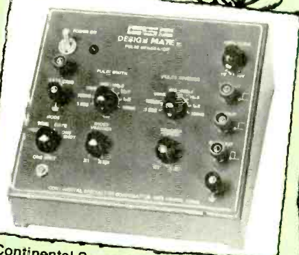
Continental Specialties "Design Mate 4" Pulse Generator
