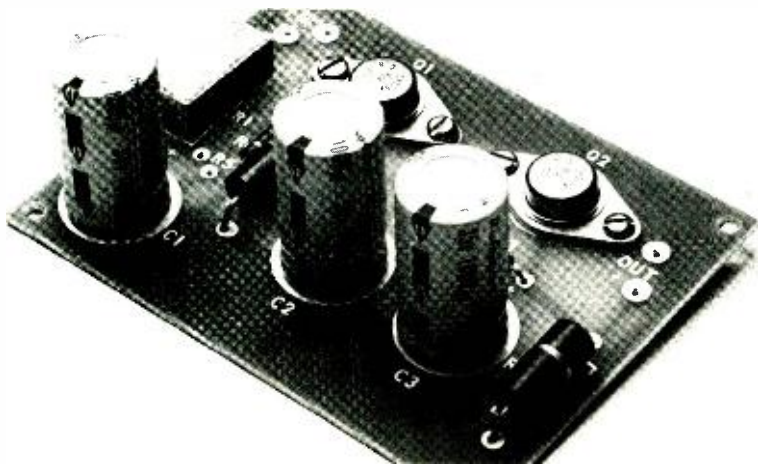
Photo shows layout of author's prototype filter.
