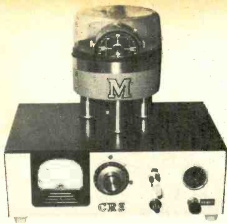
Fig. 2. Sky magnetometer remote sensor (right) and electronics package (above), into which the author has also installed a compass sensor described in Fig. 3.
