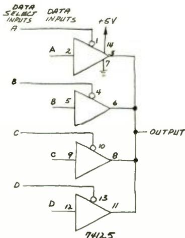
Fig. 3. Three-state multiplexer.
