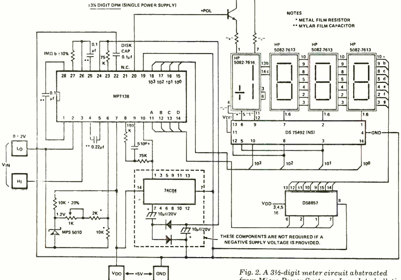
Fig. 2. A 3½-digit meter circuit abstracted from Micro Power Systems, Inc., data bulletin.
