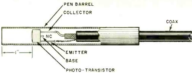
Fig. 4. To make probe, phototransistor is mounted in an old pen barrel and connected to a coaxial cable.
