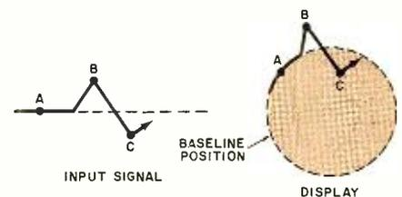
Fig. 2. Converter changes input (left) into circular display.
