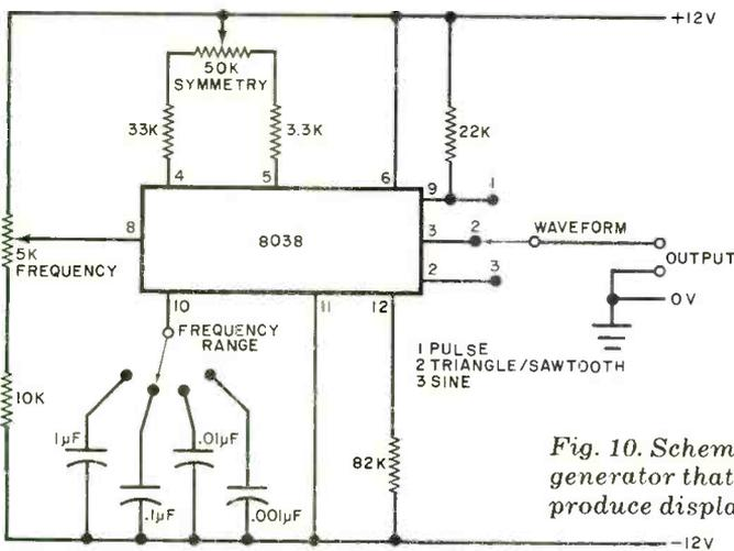
Fig. 10. Schematic of waveform generator that can be used to produce displays shown here.
