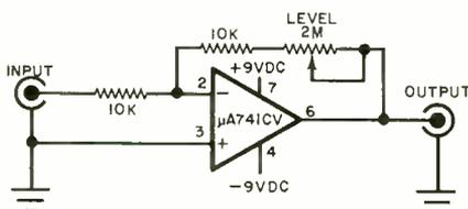
Fig. 9. Schematic of a suitable preamplifier circuit.
