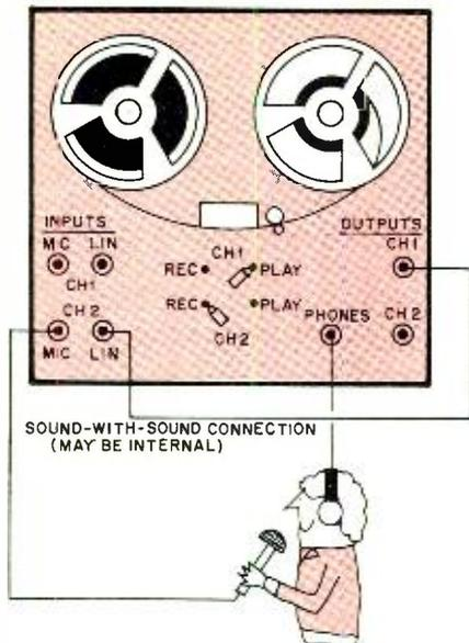
Fig. 4. Hookup for a simple sound-with-sound system.
