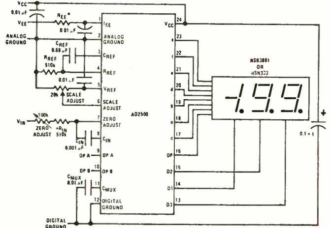
Fig. 1. Simple 2½-digit meter circuit suggested by National Semiconductor.
