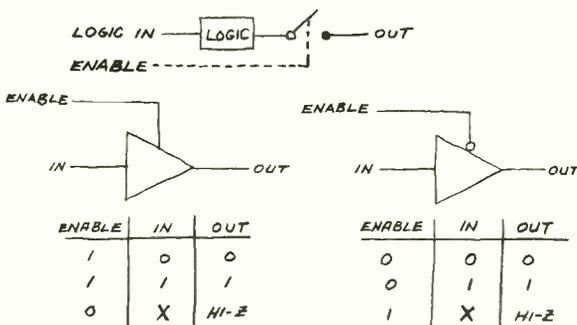
Fig. 1. Two three-state buffer configurations (left).
