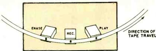
Fig. 1. Diagram shows arrangement of heads on a three-head deck.
