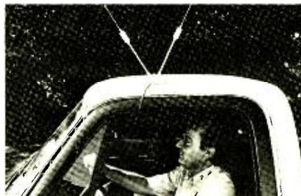
manufacturer. The twin-loaded radiating elements form a centerfed dipole with a claim of high efficiency. The antenna comes with a 6-pole magnetic base mount that measures 4" in diameter. \$21.95.
