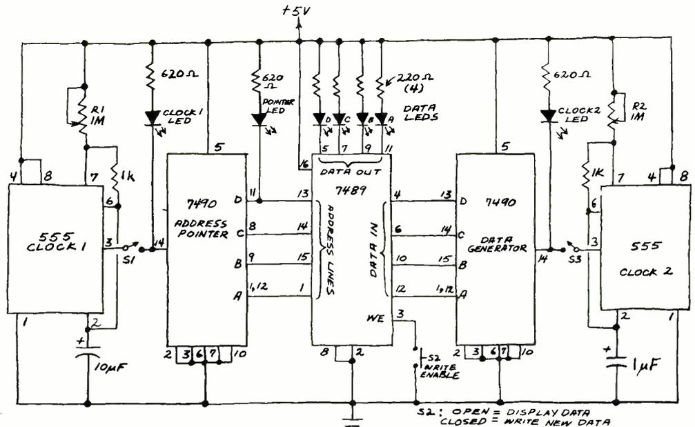
Fig. 3. Automated RAM demonstrator with pseudo-random data generator.
