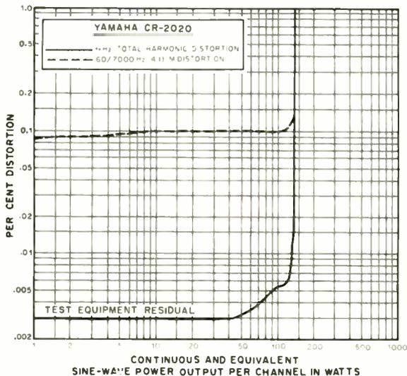
1000-Hz total harmonic distortion and 60/7000-Hz IM distortion.
