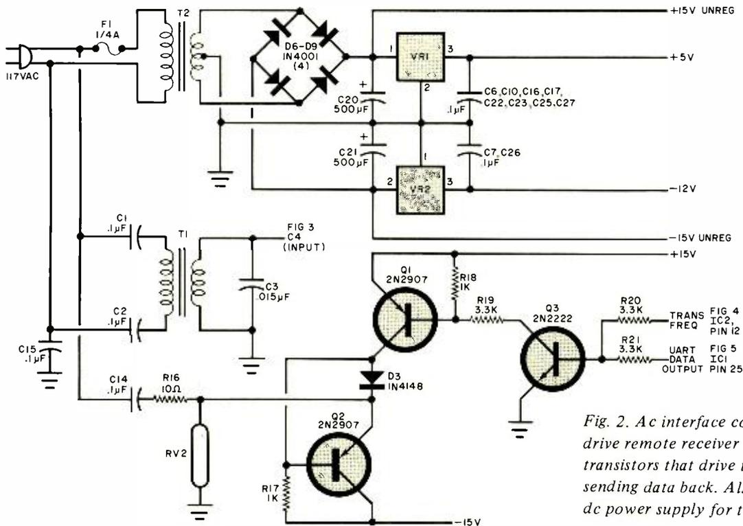
Fig. 2. Ac interface consists of T1 to drive remote receiver and three transistors that drive the ac line for sending data back. Also shown is the dc power supply for the remote.
