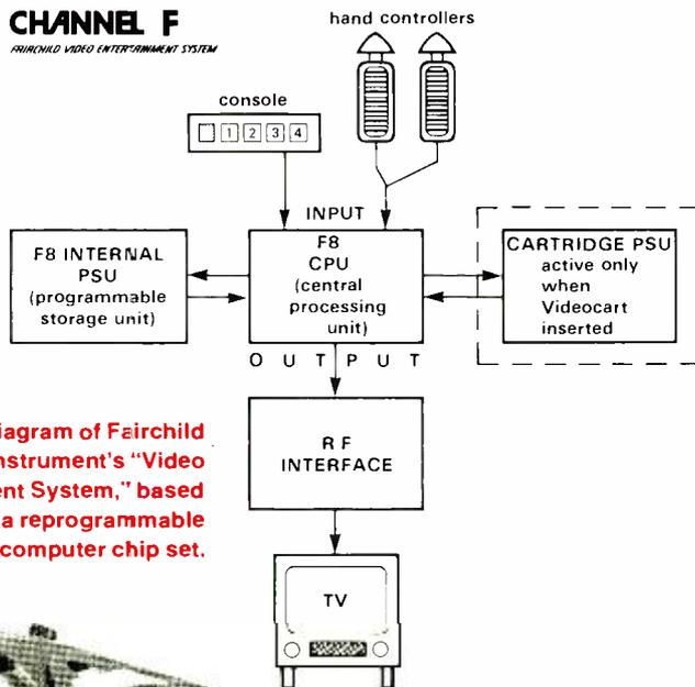
Block diagram of Fairchild Camera and Instrument's "Video Entertainment System," based on a reprogrammable microcomputer chip set.
