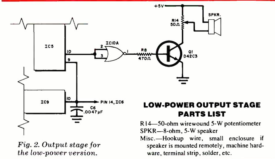
Fig. 2. Output stage for the low-power version.
