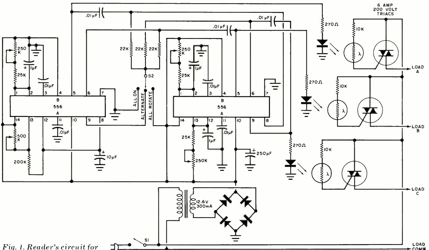
Fig. 1. Reader's circuit for flashing a string of lights.
