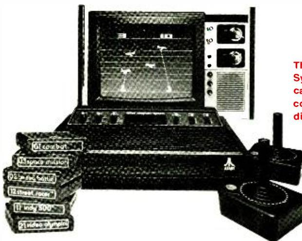
The Atari Video Computer System uses plug-in game cartridges, has two joy-stick controls, and includes a difficulty option switch.
