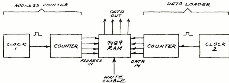
Fig. 2. Block diagram of pseudo-random data loader.
