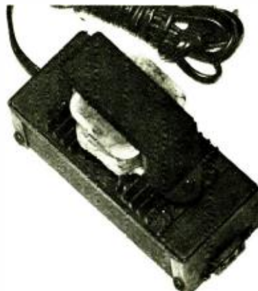
Fig. 4. Photo of assembled prototype shows transformer mounted on heat sink.
