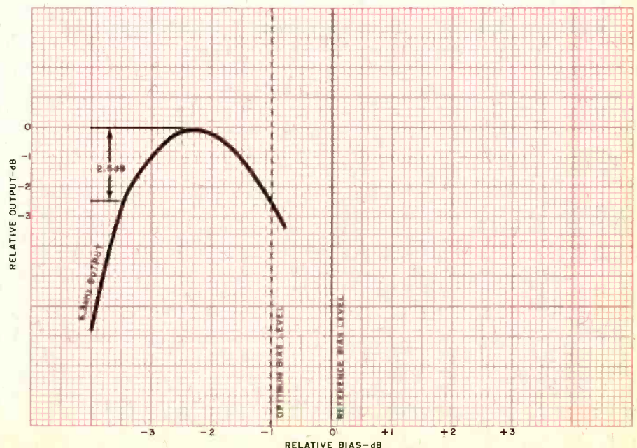
Fig. 1. Determining the bias level for a sample low-noise tape.
