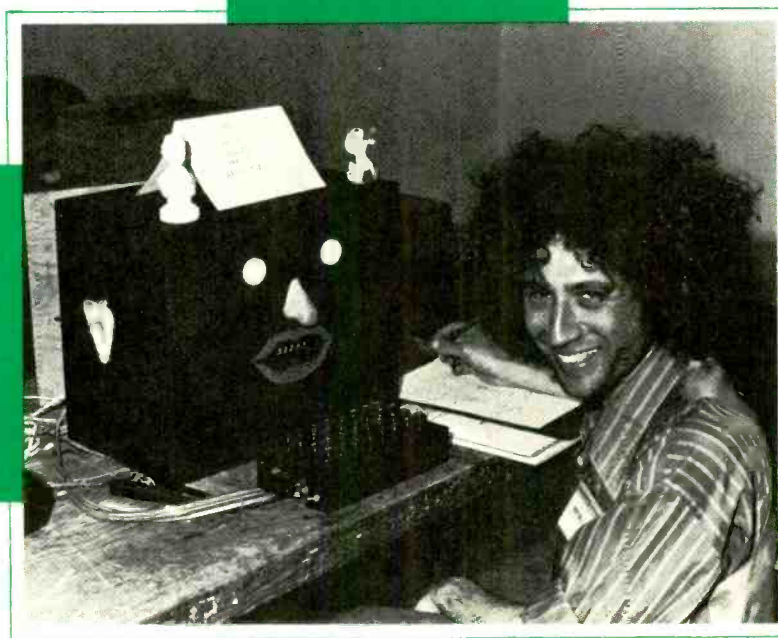
6 Rich Gold's "Mr. Computer" is based on a KIM-1 and 200-byte program. Its coded messages (via LED displays in its mouth) are interpreted by Rich in storybook form. He plans to add video graphics and electronic music output.
