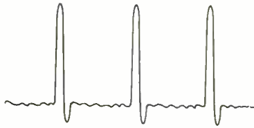
Fig. 2. Trumpet waveform miked on axis in anechoic chamber. From a Denon record made with pulse-code-modulation process.
