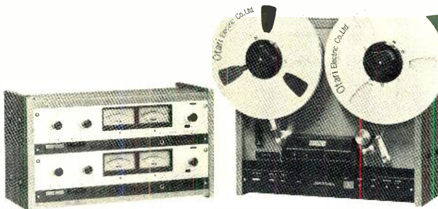
The Otari MX-5050-QXH has "Sel/Rep" for recording two discrete but time-synchronized tracks.
