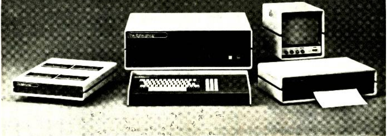
Clockwise from top: CPU, Video Monitor, Impact Printer, Keyboard, Cassette Storage System with Four Drives
