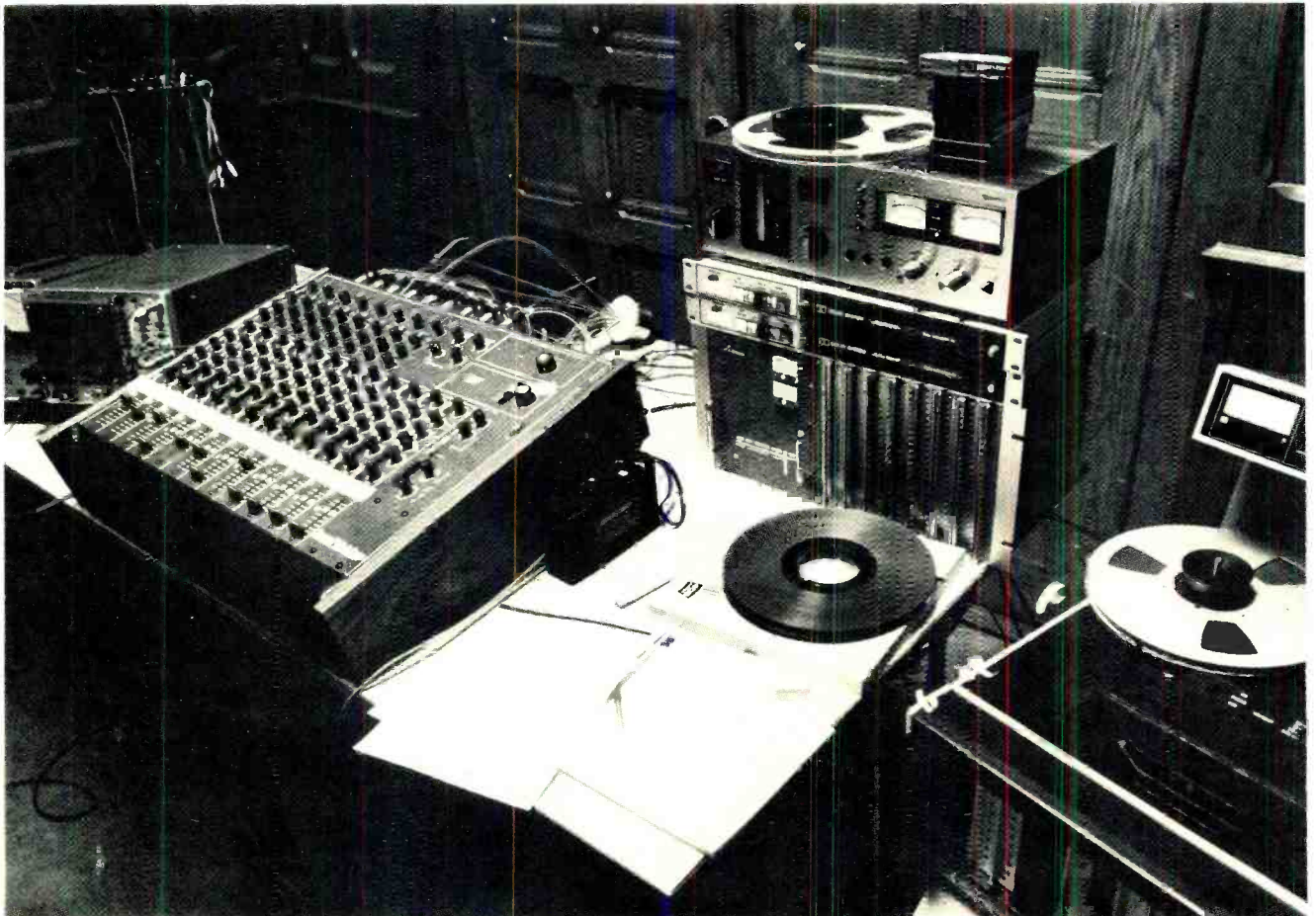
The control-room setup, showing the console, a corner of the tape transport (right), the scope and voltmeter (far left), and the mysterious cassette deck.
