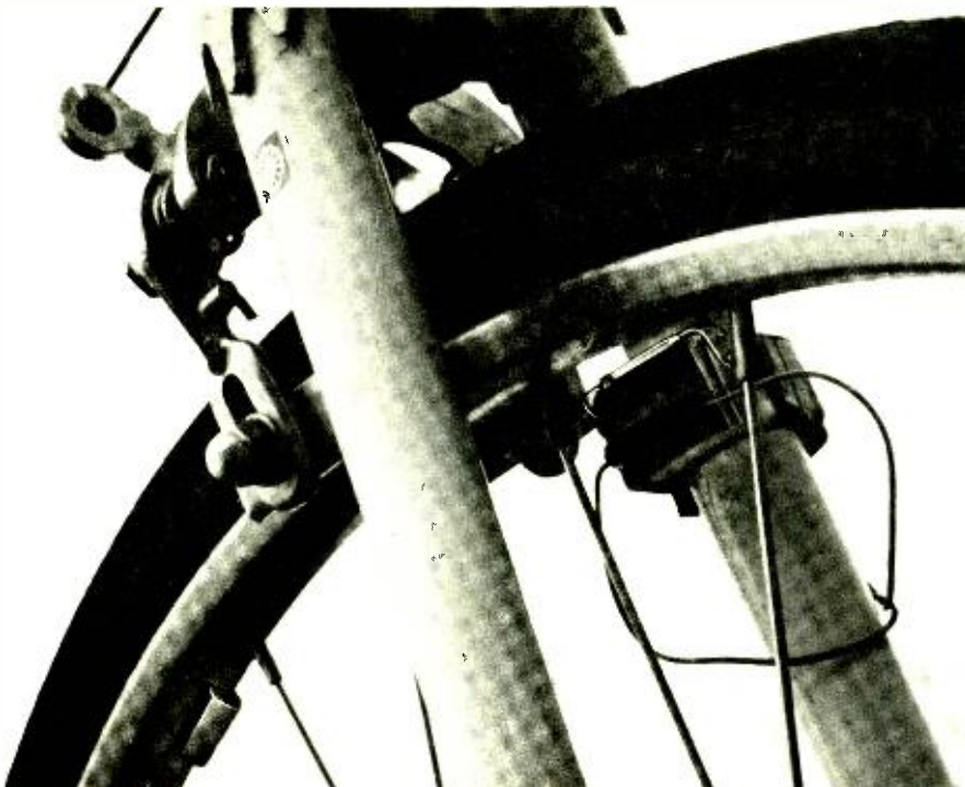
Photo shows how reed relay is clamped to fork holding front wheel of bicycle with magnets (one shown) on inner rim.
