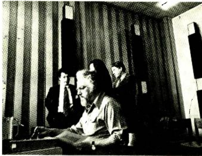
Fig. 2. The Acoustic Research Digital Time Delay System, showing six of the sixteen speaker channels and a side view of electronics.
