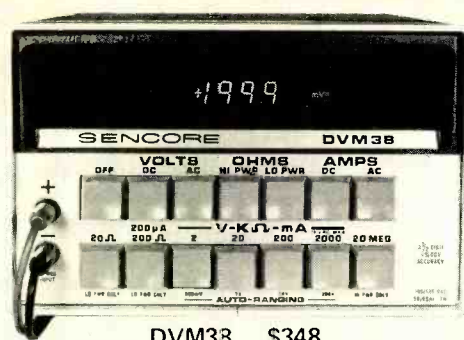
DVM33 $348 3½ digit LED display, .1% DCV accuracy, AC operated, auto-ranging, auto-zero, king size pushbuttons
