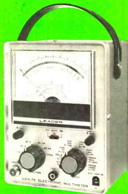
The Leader Model LEM-75, a transistor multimeter, has a temperature scale that is used with an accessory probe.
