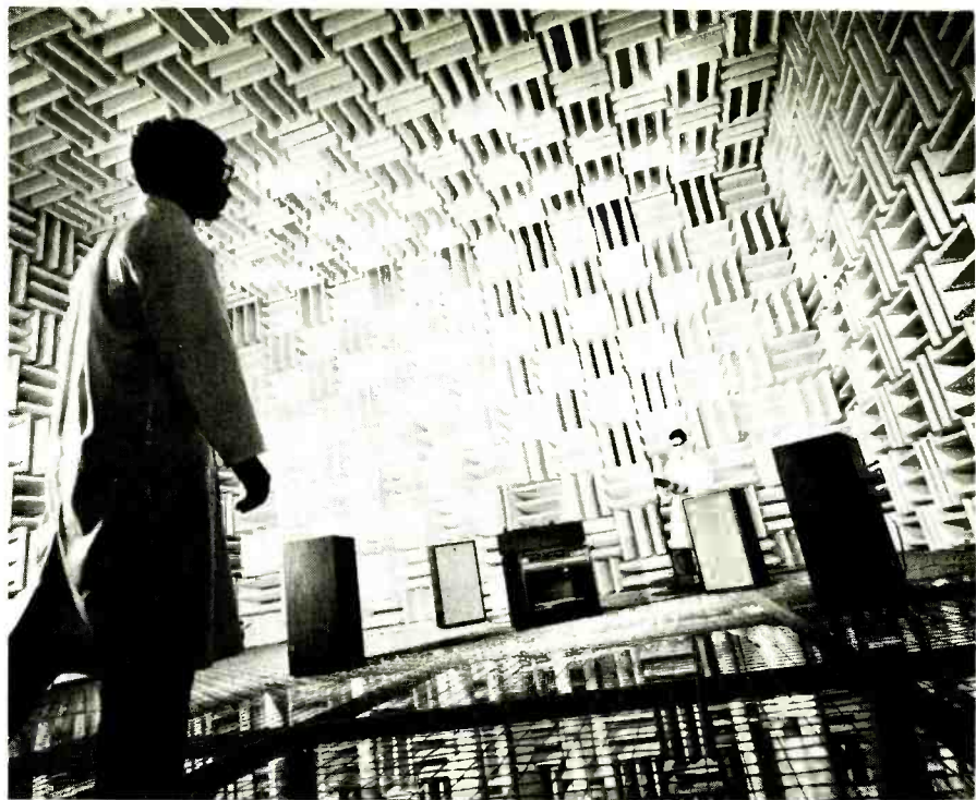
Fig. 2. JVC's unusually large anechoic chamber.
