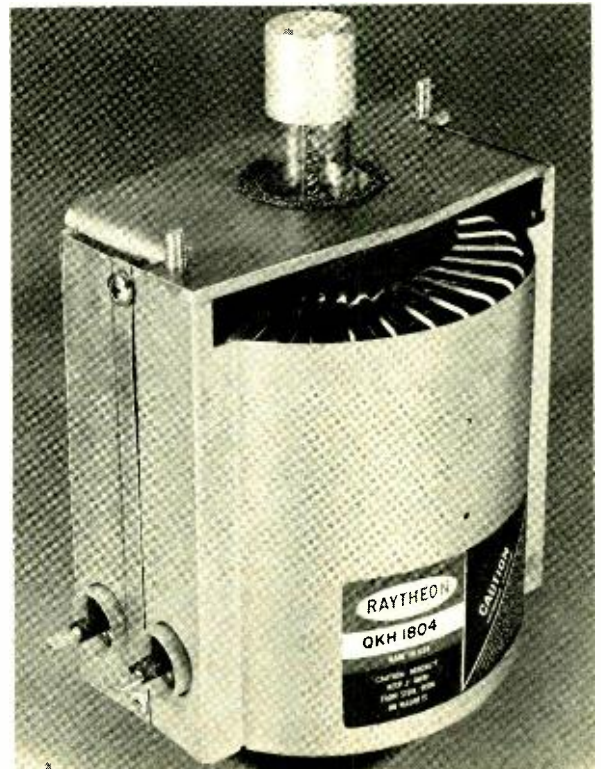
Typical magnetron tube is housed in rugged metal container along with necessary magnets.
