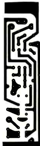
Fig. 2 Actual-size foil pattern and component installation on a board that can fit a 7/8" ID tube. The positive battery clip is soldered to one end of the board, with wire connection to the negative terminal.
