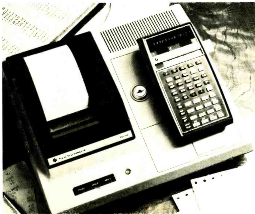
Ti's PC-100 desktop cradle was designed for use with either the SR-56 or SR-52 calculators.
