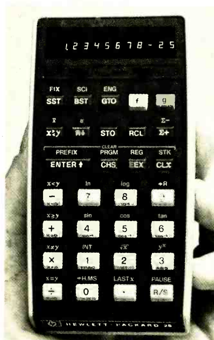
The HP-25 is smallest programmable. Has 49 program steps, 8 conditional comparisons and full editing.
