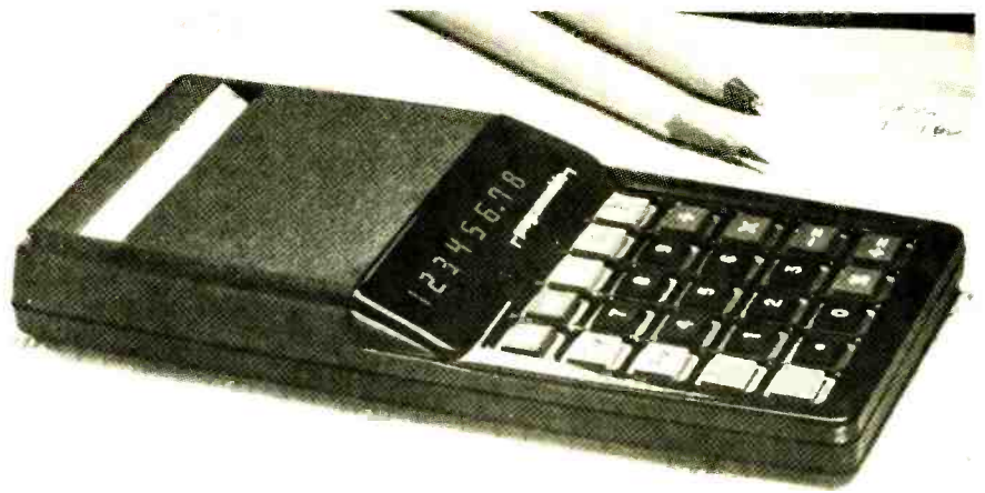
The Litronix Model 2290 features a 10-step program memory and data memory to facilitate complex repetitive problems.
