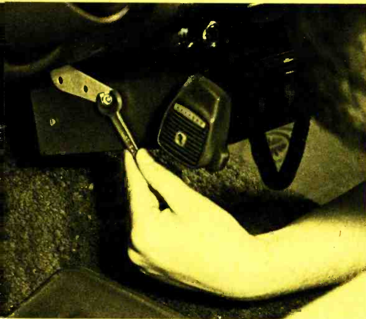
2 Mounting transceiver under dash.
