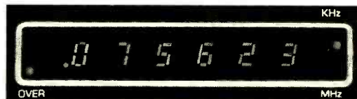
KHz display of same CB channel showing suppression of leading digits.
