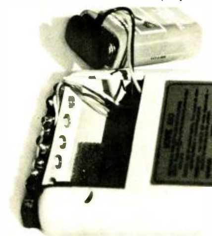
Arrange wires in battery well so they do not interfere.
