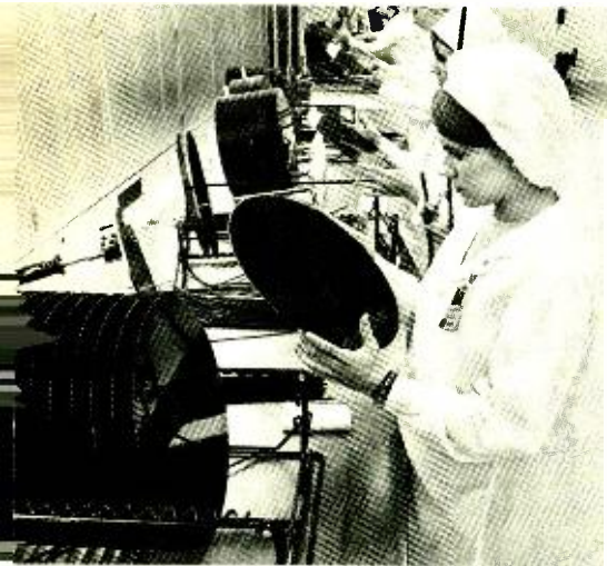
Fig. 2. After coating, steps are carried out under clean-room conditions, including inspection.
