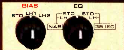
Selectable equalization and bias switches.
