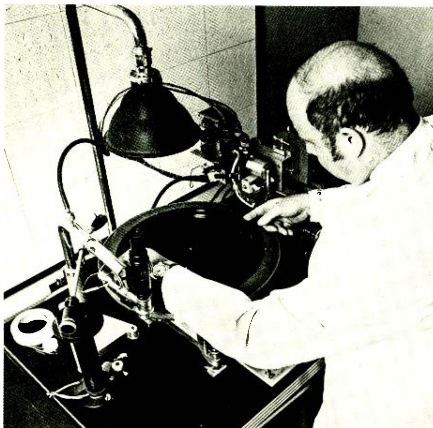
Fig. 1. Disc-cutting lathe used for evaluation of lacquers. Test cuts can be seen on the lacquer's surface.
