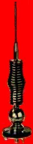
MODEL 2-202. MOBILE ANTENNA. 102" stainless steel whip. Stainless steel spring. 180° swivel mount. All hardware included.
