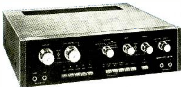
Four-channel versatility is represented by Lafayette Radio's LA-74 built-in Full Logic Wavematching SQ and other matrix decoding, with demodulator provisions for CD-4 (below).
