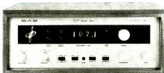
Digital readout FM tuning sections, as in SAE'S Mark VIB FM stereo tuner, exhibit growing popularity (below).
